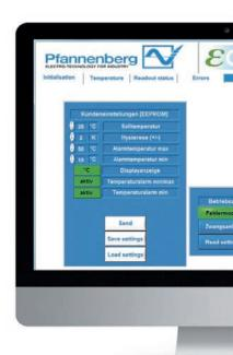
Plant is the Pfannenberg system software with which you can not only read out status information of cooling units, but also set and adjust parameters. There is the possibility to communicate directly with the cooling units or to incorporate the software into the user interface of your machine control.
