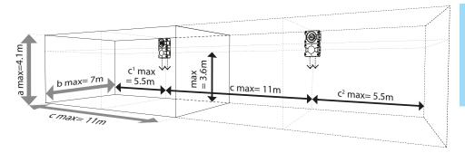
Signaling ranges of the PATROL flashing light sounder PA X 1-05, 24 V DC, clear lens, using the example of wall mounting.
