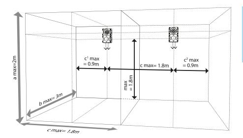
Signaling ranges of the PATROL flashing light sounder PA X 1-05, 24 V DC, red lens, using the example of wall mounting.
