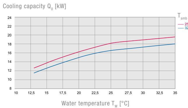
The performance curves do include standard pump losses and refer to 50 Hz and 20 % glycol mixtures.
