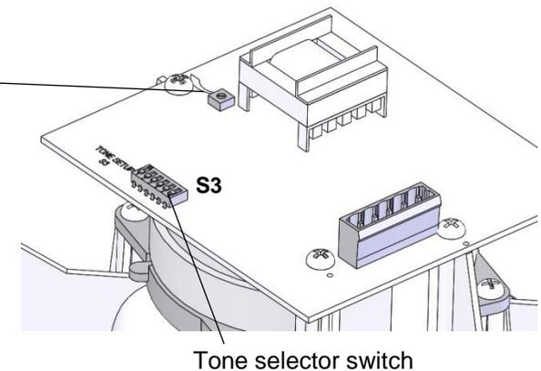
The desired tone can be selected using the **S3** tone selector switch. The tone is generated after the supply voltage is applied. A complete tone type table can be found in the Annex. See the digital operating instructions for the external control of other tones, source: [www.pfannenbergl.com/manuals](http://www.pfannenbergl.com/manuals).
