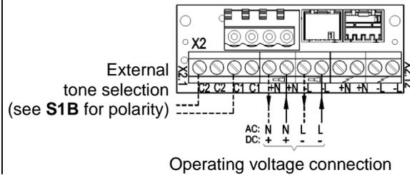
Separate connection of flashing light and sounder
