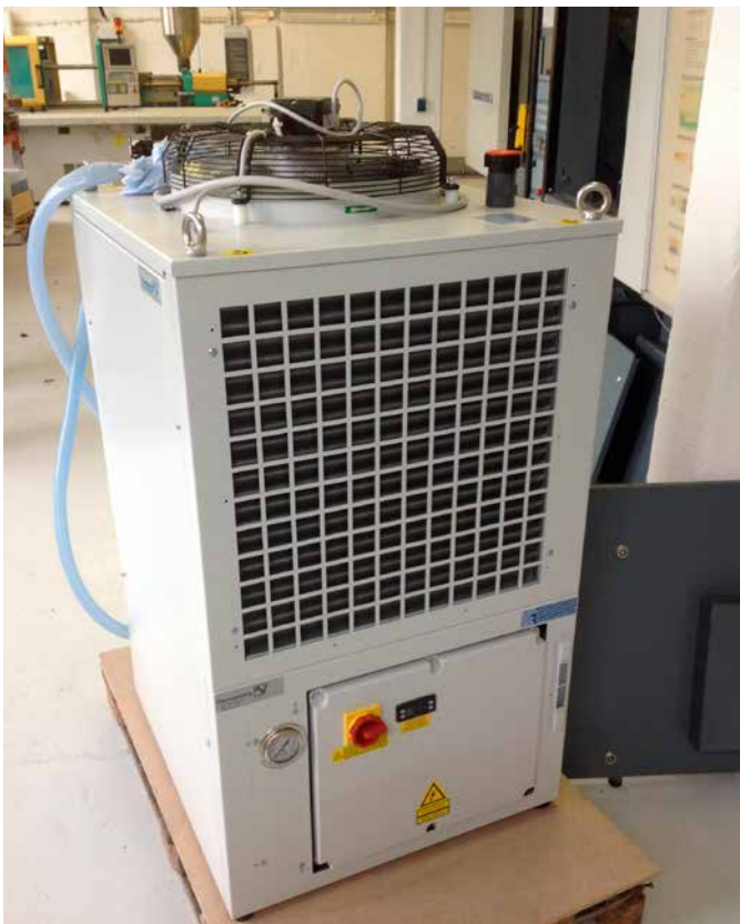
A type EB 130 WT CE STD chiller cools the injection moulding process of three injection moulding machines
