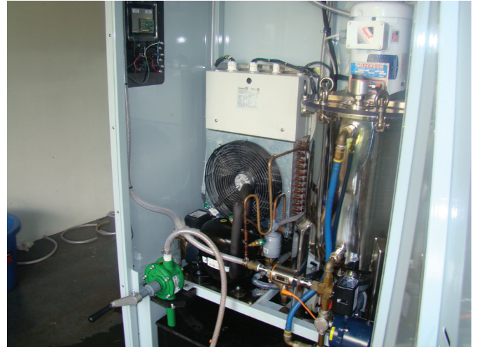
Pfannenberg open-frame chiller inside packaged Ferrator.
