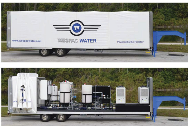
Pfannenber chillers on trailer-mounted Ferrator.
