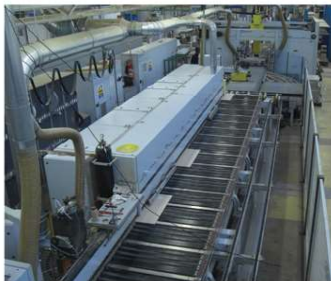
The edge banding machine in Duravit's Schenkenzell plant runs about 4,500 passes a day.
