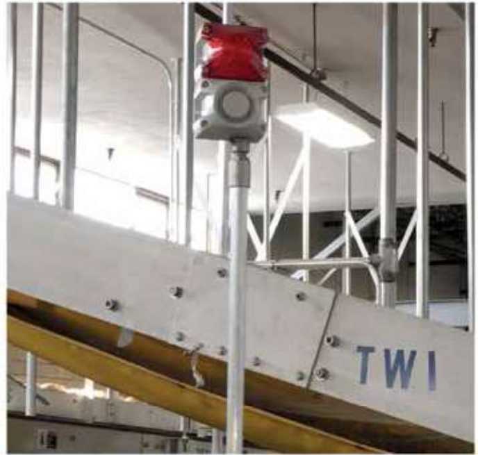
Pfannenberg PA X 1-05 100 dB Flashing Light Sounder attached to inspection machine
