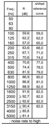
Evaluation as per ISO 717-1  $R_{w}$  (C,C<sub>tr</sub>) = 78 (-2;-7) dB
