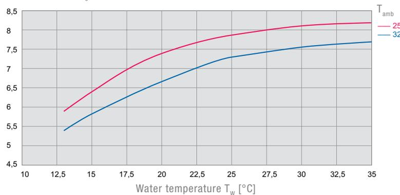
The performance curves do include standard pump losses and refer to 50 Hz and 20 % glycol mixtures. For a 40 °C ambient temperature you can expect capacity values shown for 32 °C to decrease by 20 %. For a 45 °C ambient temperature you can expect capacity values shown for 32 °C to decrease by 30 %.
